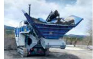
**The MOBICONE MCO 90i EVO2's feeding unit is compact and equipped with a simple sliding mechanism.**
