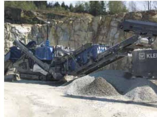
**The MOBICONE MCO 90i EVO2 features the innovative D-DRIVE "diesel-direct-electric" drive concept - making it both powerful and economical.**
