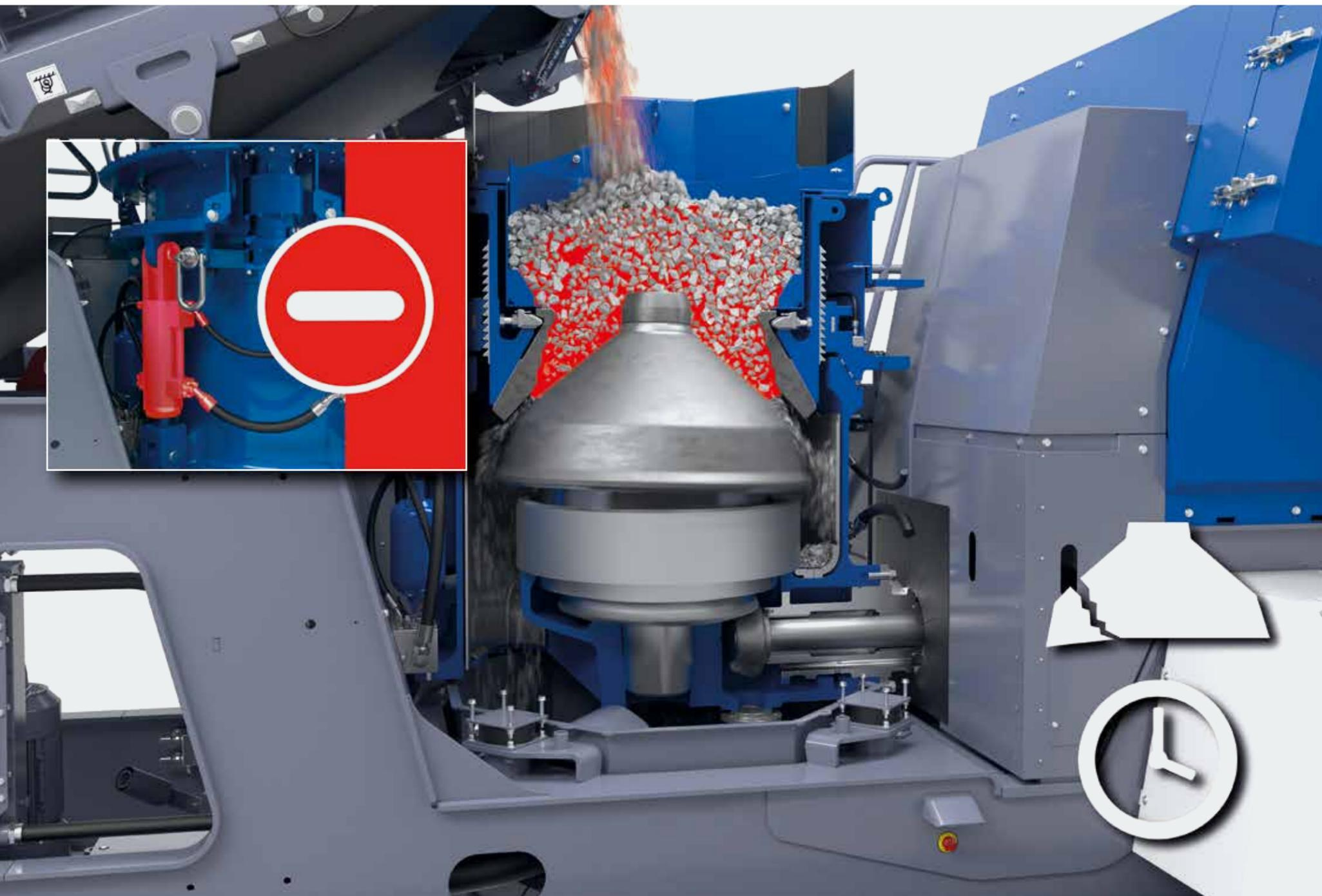
Additional overload detection is provided by the intelligent "Ringbounce Detection". Here, the hydraulic pressure and other parameters of the crusher are continuously monitored. If necessary, the system reacts and prevents latent overloads that could cause serious damage.
